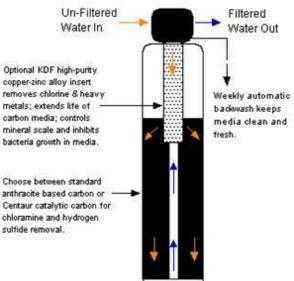
Filter Tank sizes depend on water flow requirement to the house, Villa, or complex.
