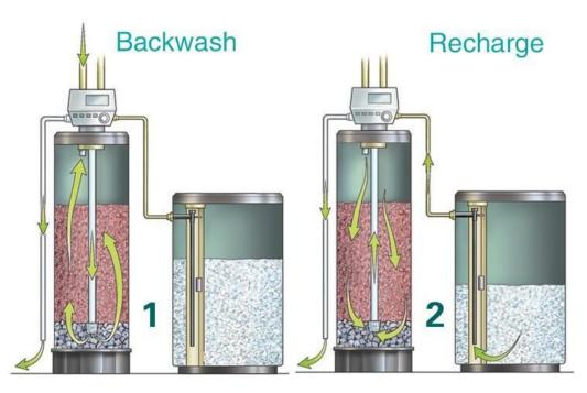
**SMART** Ion Exchange Softeners use a High Capacity Cation Softening Resins. When the water flows over these negative charged resin Ions, the Ions attract (like a magnet) the positive charged minerals & metals in water to reduce the hardness and improve the water quality
